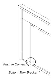
Completely secure the full screen door to the unit by securing 4 screws to the Left and Right Side Trims.
